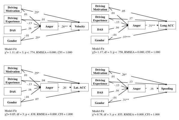
Figure 2: Path models for personal characteristics, reported anger and driving parameters (velocity, longitudinal acceleration, lateral acceleration and speeding) in the first study. p < .05; \*\* p < .01; \*\*\* p < .001
