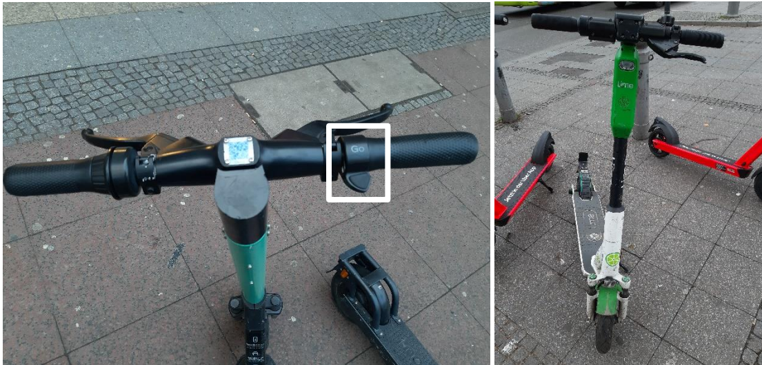
122 Figure 1. Handlebar of a Tier e-scooter equipped with two hand-lever brakes and a highlighted 123 acceleration thumb-lever (left) and Lime scooter with single left-hand lever brake and foot brake for 124 the back wheel (right).
